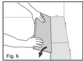
\* Locking pins in first row can be engaged as second row boards are installed, however best results may be obtained by using method 1 or 2, thereby locking first row boards as you go.
